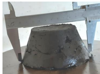
Figure 3. Flow of fresh mortar geopolymer.
